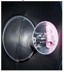
D. Connect the 3/8 inch tubing by removing the compression fitting from the elbow.
